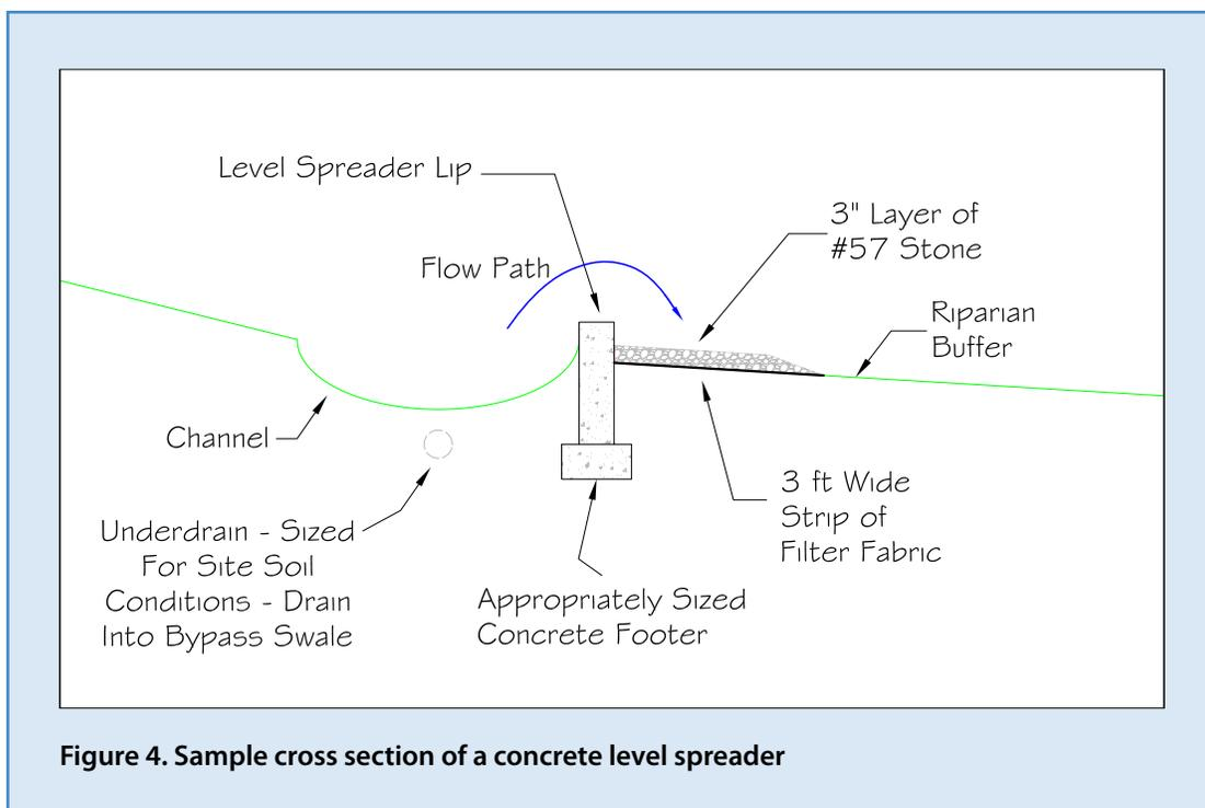
**Figure 4. Sample cross section of a concrete level spreader**
