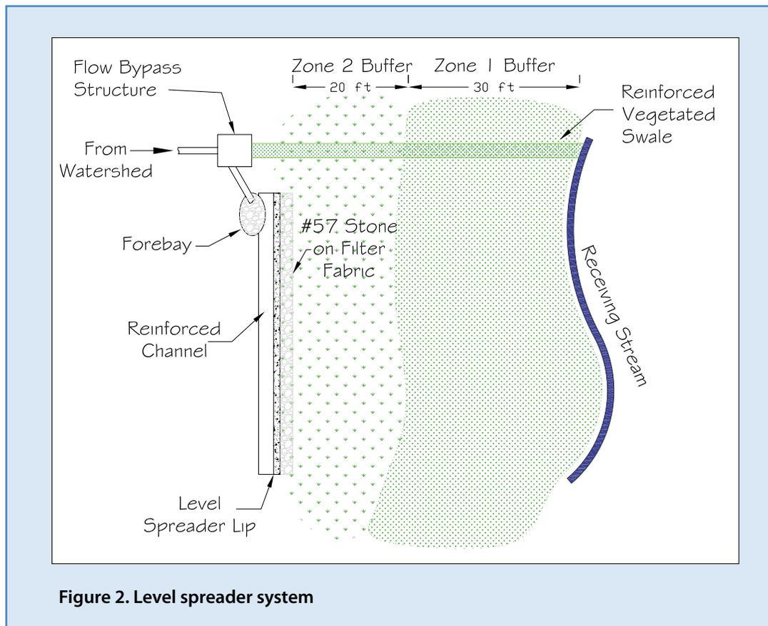
**Figure 2. Level spreader system**
