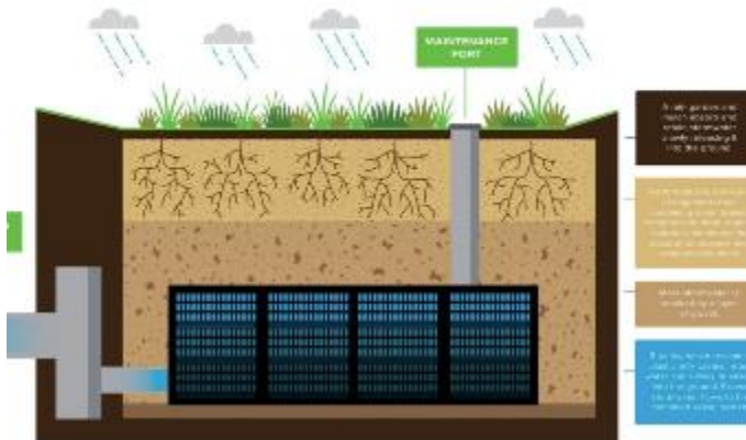
Layers and Cross-Section of a Bio-Retention System
