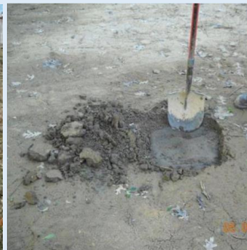
Clogged Filter Bed
