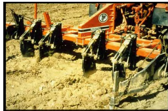
Fig. 13. The same deep, angled-leg subsoiler shown in Fig. 7 is engaged at maximum depth for Phase 2, decompaction (deep soiling), of the replaced topsoil and the upper subsoil materials.
