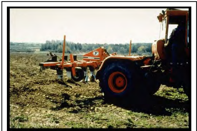
Fig. 8. A deep, angled-leg subsoiler, ideal for Phase 2 decompaction of after the topsoil layer is graded on top of the ripped subsoil.
