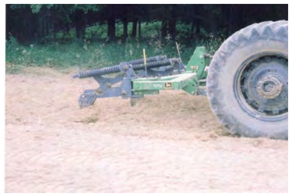
Fig. 11. A repeat run of the 3-shank ripper along the same patterned pass area as Fig. 9; here, incrementally reaching 18 of the needed 22 inches of subsoil fracture.
