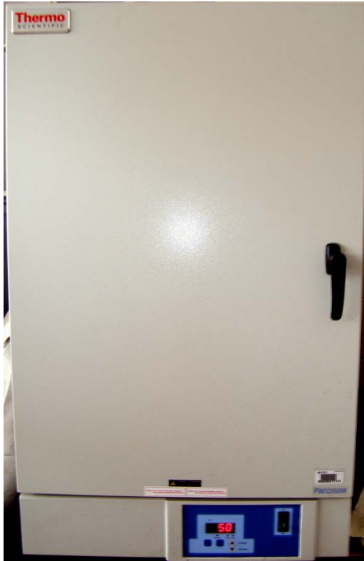
Figure 2: Oven set to 50 to 60 degrees C for drying out the collected sample placed in Pyrex dishes
